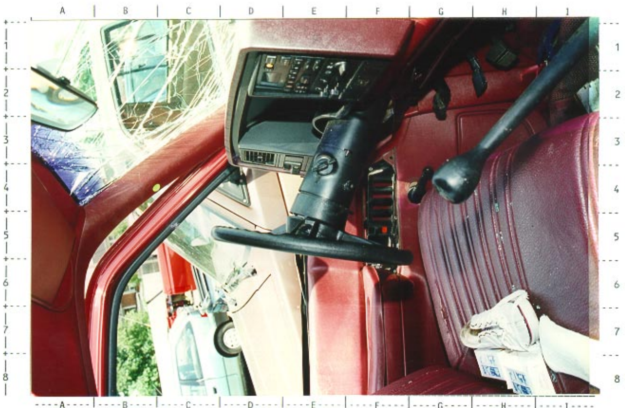
# 84 -- Deformed steering wheel in 1988 Chevrolet C-1500 pickup viewed from right front passenger side
